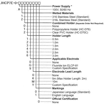
\* Power for the cleaning system is provided through the transmitter. When operating with power supplies other than 100V, a step down transformer must be separately purchased (Model ZP, 35VA).
