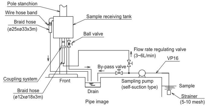
● Sampling type (mounted on aluminum frame)
