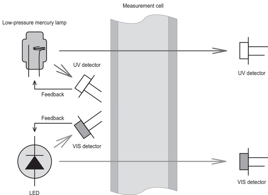
The OPM-1610 uses the dual wavelength technique to measure pollutants. This technique adopts two highly stable sources of light, UV (ultraviolet) and VIS (visible light).
