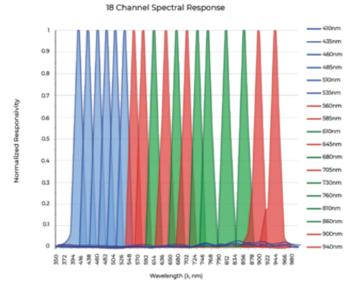
18 wavelengths throughout the UV - VIS - IR range are covered by sensors used by the PrimeLab 2.0. Narrow peaks on the spectral curve allow utmost accuracy.
