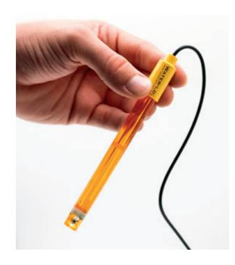
PrimeLab 2.0 has the option to connect test probes, such as those used for pH, EC, TDS, Salinity, ORP and Temperature. By connecting probes to the PrimeLab 2.0, the photometer manages the probe, obtaining readings which can be stored under the user-defined sampling points and synchronized to the LabCOM®-Cloud (optional).
