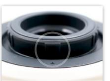
Step 3: Please make sure that the raised area on the adapter is in line with the traingle\*/arrow on the PrimeLab 2.0
