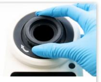
Step 2: Turn the adapter clockwise until you hear and feel the adapter click into place.
