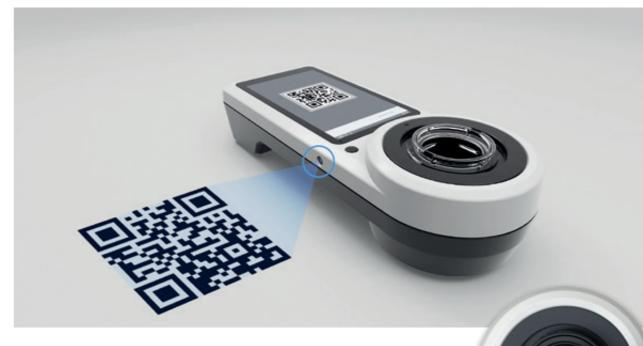
With the built in camera, the PrimeLab 2.0 gives the option to scan QR-codes to identify sampling points set up by the user and to identify reagents with QR-codes on the package. The advantages of this options are significant:
